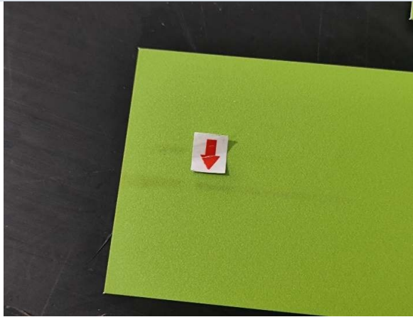
Photo 3: Hanging strip, dirt mark
